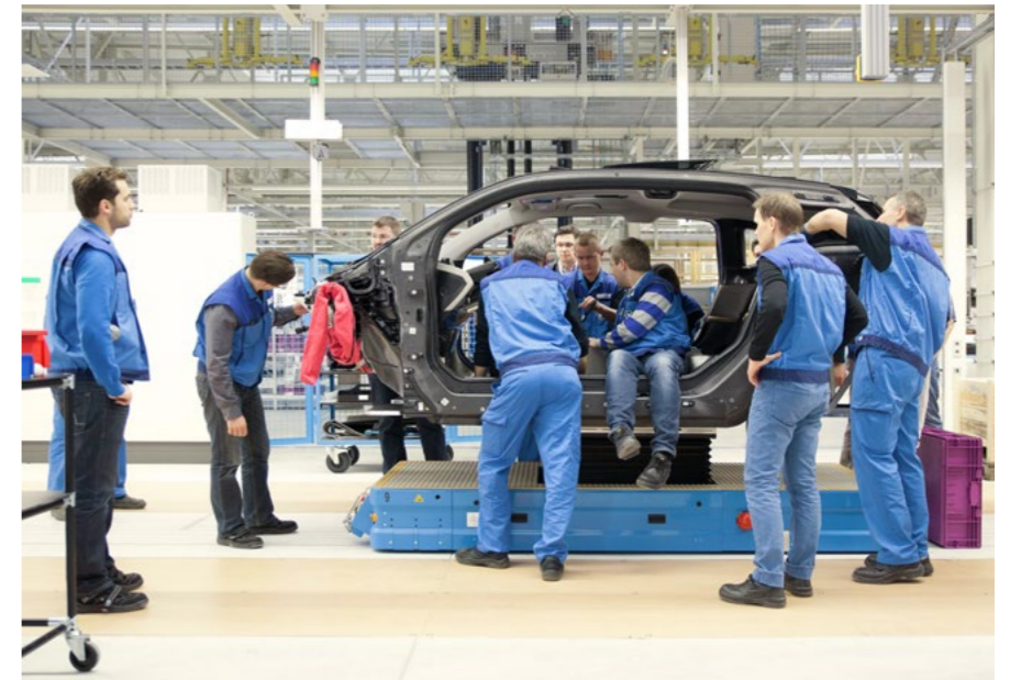
Modern lightweight design: the carbon-fibre frame for the production of the BMW i3 at the BMW Group plant in Leipzig.
