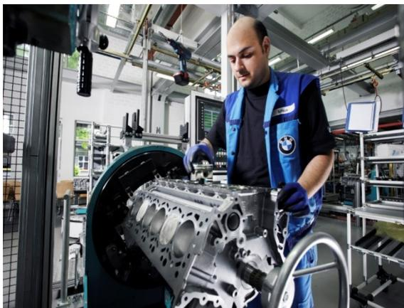
The light metal foundry at the Landshut plant produces engine core components such as crankcases and cylinder heads, which are then further processed in mechanical production. Landshut and Dingolfing also produce the electric motors, range extenders, and high-voltage accumulators as well as engine-gearbox units for BEV and PHEV models.
