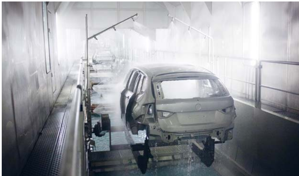
PAINT SHOP AT THE BMW PLANT LEIPZIG — Innovations lead to gradual introduction of wastewater-free production processes.
